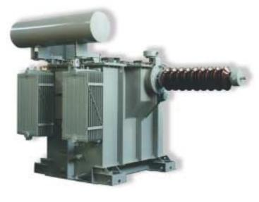
Earthing transformer for limitation of short-circuit current to earthfault. 24 MVA/10 s – Single Phase – 76 kV/8 kV-60 H<sub>2.</sub> Extremely robust design (both electrical and mechanical).
